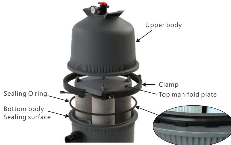
Figure 6 The fluted side of the rubber Sealing O ring face down
