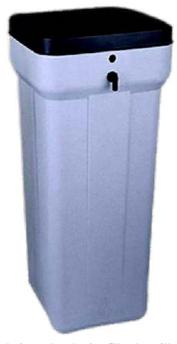
The brine tank is filled with salt tablets or flakes immersed in water to dissolve slowly to provide bribne (very salty water) that is drawn through the resin at regular intervals to regenerate it.
