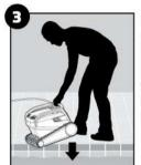
Put the pool cleaner in the pool and let it sink to the floor. Make sure that the floating cable is free of any obstructions.
